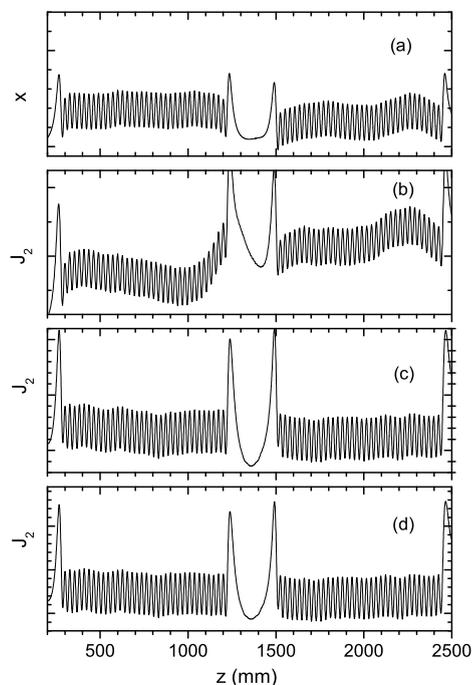
**Fig. 1** Path  $x(z)$  of a 20 MeV reference electron through the two units of the U27 undulator (gap  $g=15$  mm) calculated on the basis of a Hall-probe measurement (a) and second field integrals  $J_2(z)$  determined by means of the pulsed-wire method before (b) and after (c) shimming several undulator magnets. Fig. (d) shows the field integral measured for the smaller gap  $g=13.5$  mm with the same shimmed magnets.
