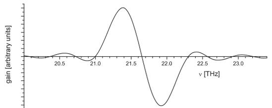
**Fig. 4** Single-pass gain versus frequency  $\nu$  calculated for 0.1 V/m initial field strength and 100 macro-particles representing a monoenergetic electron bunch with a charge of  $Q = 50$  pC and 20 MeV kinetic energy.
