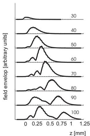
**Fig. 1** Envelope of the radiation field at the undulator exit after 30, 40, ..., 100 passes calculated for one unit of the U27 undulator of ELBE (parameters see table 1 of ref. [4]). The resonator detuning is  $-0.5\lambda$  and 5% round-trip loss has been assumed.
