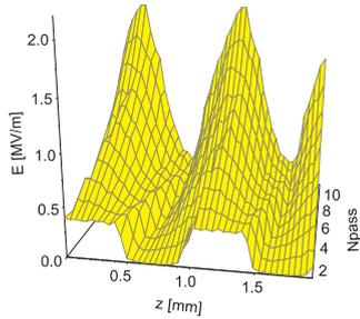
**Fig. 1** Amplification of a wavetrain during 20 passes in a FEL. The radiation is modeled with 20 ( $N = 21922$ ) modes. The corresponding pulse repetition frequency is obviously too high; The radiation pulses overlap.
