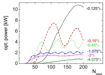
but saturates at a higher power level which is characterized by remarkable oscillations. Detuning the resonator stronger than the value of optimum gain leads to both a small gain and a lower power level at saturation.
