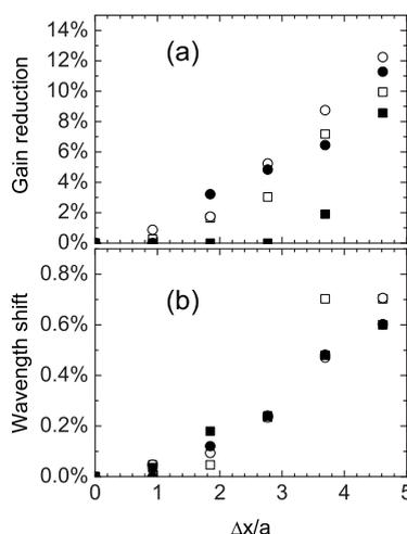
**Fig. 3** Gain reduction (a) and wavelength shift (b) as a function of the ratio  $\Delta x/a$  (defined in fig. 2) calculated for a 20 MeV (open symbols) and 40 MeV (full symbols) electron pulse. The squares and spheres, respectively, represent a calculation without and with beam emittance (15 mm\*mrad, 50 ps\*keV) taking into account.
