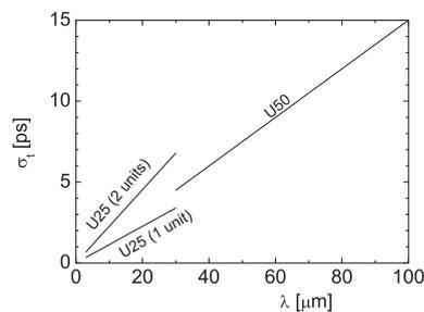
**Fig. 4** Electron pulse lengths  $\sigma_t$  corresponding to the condition  $\mu_c = 1$  is a function of the laser wavelength calculated for the undulators of ELBE.
