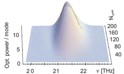
**Fig. 3** Internal laser power as a function of the longitudinal coordinate  $z$  and the number of passes  $N_{\text{pass}}$
